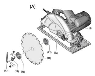
Fitting the saw blade (see figure A)
