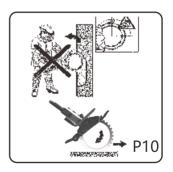
4. Oping means the incision and the saw blade. If the workpiece is not properly supported and displaced during cutting, the saw blade is clamped or stopped, and the reaction force occurs
