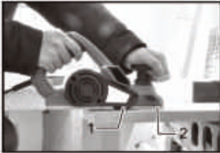
1. Blade edge 2. Cutting line
